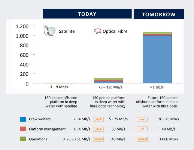
Currently, data transmission on an deep water offshore platform far from the shore is limited and constrained by its satellite connection to well below 10 Mb/s
