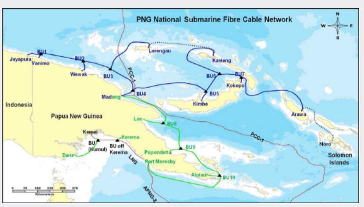
The PNG LNG Fibre cable will form part of the PNG National Submarine fibre optic cable network
